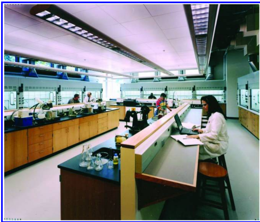
Figure 1. College of Wooster, Severance Chemistry Building: Organic teaching laboratory with bullpen configuration and perimeter fume hoods. Payette, Architect Image Credit: © Timothy Hursley. (see color insert)
