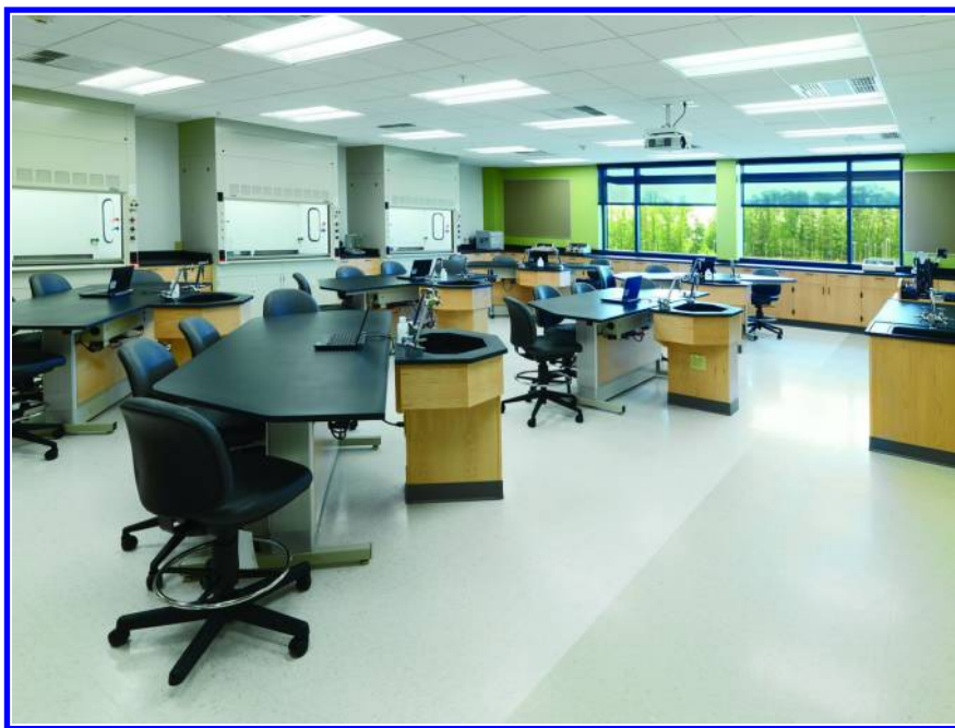
Figure 1. Fume hoods are reserved for the perimeter in this chemistry lab at John Tyler Community College. (photo courtesy of Philip Beaurline). (see color insert)
