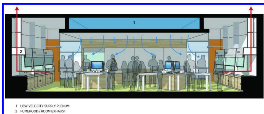
Figure 10. HVAC Diagram: Low volume supply air is distributed through a ceiling plenum over the central teaching area and exhausted through the perimeter fume hoods. Payette, Architect Image Credit: © Payette. (see color insert)
