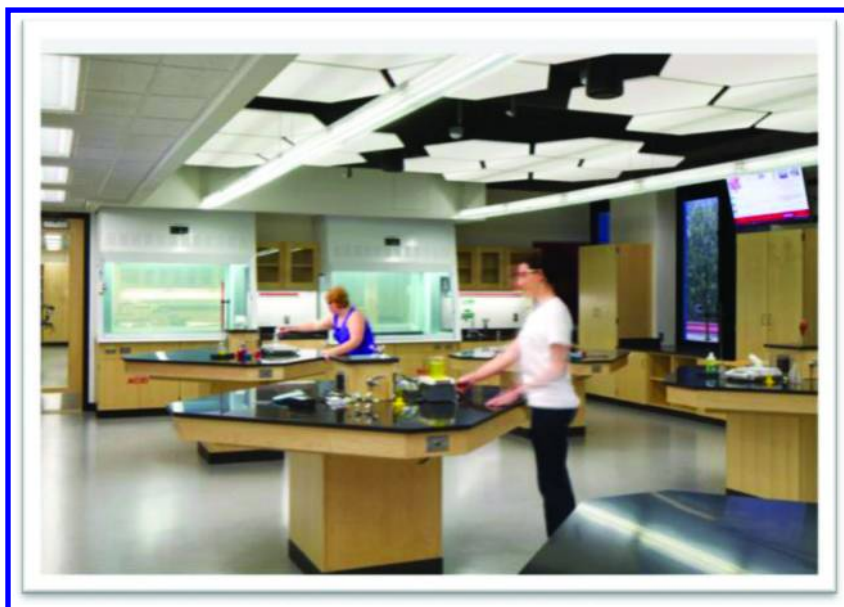
Figure 1. Island benches in the renovated general chemistry laboratory room, Spring 2012. The doghouse (small raised platform) in the center of each island bench has eight electrical outlets and two vacuum ports. Each bench has an HDMI connection to a wall-mounted large-screen monitor. Photo courtesy HDR Architecture © 2012 HDR Inc.
